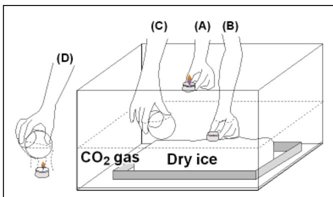
Figure. Testing for  $\text{CO}_2$  by extinguishing flame.
