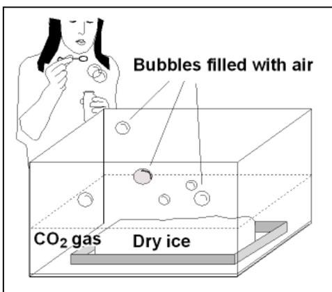
Figure. Using the property of density to test for  $\text{CO}_2$  gas that collects in the tank as dry ice sublimates.
